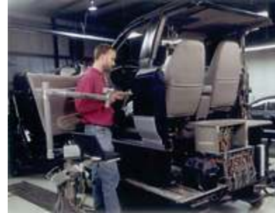
Figure 1: Components of Programmable Vehicle Model (PVM) include computer/controller that drives components of the PVM into various positions. Technician checks final position of components with FaroArm.
