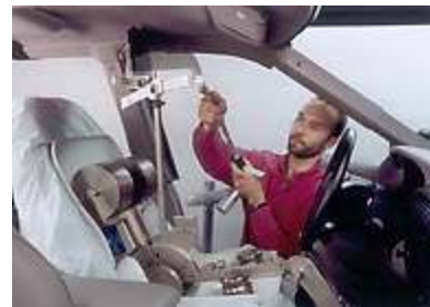
Figure 2: Technician measures headroom with FaroArm on Prefix PVM. Weights compress seat cushions to simulate that caused by a driver's body weight.
