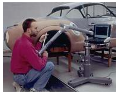
Figure 4: Technician taking surface measurements on clay model with FaroArm. Image of surface is "built" in the computer, then flipped to produce the mirror image part. Thus, by developing an image of a model's right fender, Prefix can quickly create the image of the mirror image left fender.
